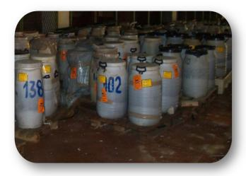
Another sewage sludge contaminated with mercury are created by washing work wear and cleaning of working space is stored in plastic barrels and there are 62.4 t waste at the moment in factory.
