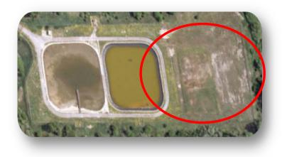
Sewage sludge from production process (the electrolyte decanting process) contaminated with mercury (in ppm concentration) was disposed at engineered landfill (from 90s) in the factory. There are now 5284 t of sewage sludge contaminated with mercury in two landfills; HDPE foils is used.
